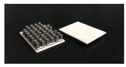
TEGs are a 'high impedance' voltage source
